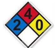
Appearance: Colorless Physical Form: Gas or Liquid (Under Pressure) Odor: Odorless (or skunk, rotten egg or garlic if odorant added) NFPA 704 Hazard Class: Health: 2 (Moderate) Flammability: 4 (Extreme) Instability: 0 (Least)
